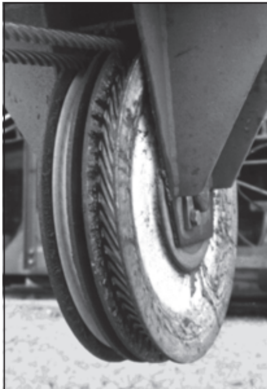
Figure 1: Wire rope sheave with negative impressions
