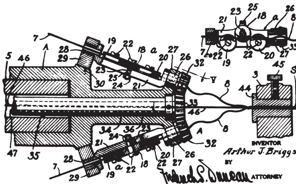
Fig. 17: Briggs' preforming head with rollers
